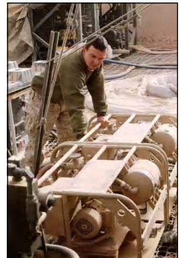
A water purification technician with 8th ESB turns on a water pump at Forward Operating Base Nelay to supply water for laundry and shower services for 3d Battalion, 5th Marines (3/5) in the Sangin District of northern Helmand Province.
